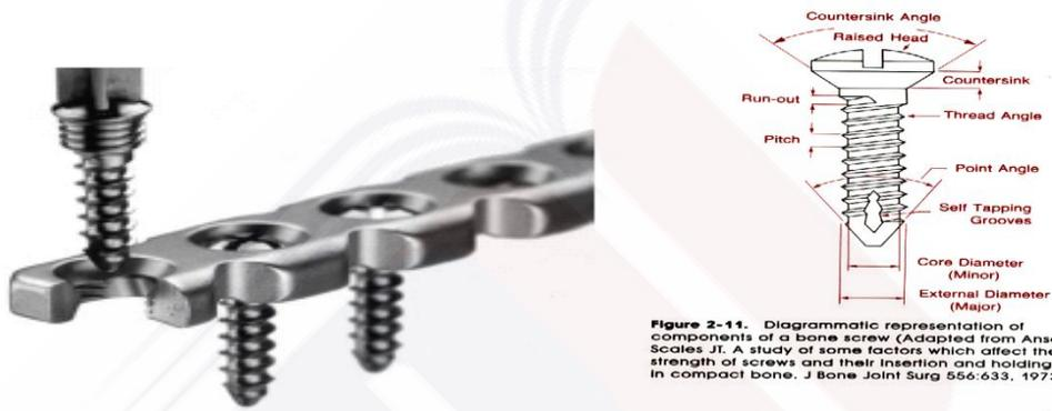
Figure 2-11. Diagrammatic representation of components of a bone screw (Adapted from Ansell RH, Scales JT. A study of some factors which affect the strength of screws and their insertion and holding power in compact bone. J Bone Joint Surg 55:633, 1973).
